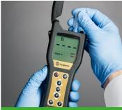
2. Snap swab & insert into ATP Meter
